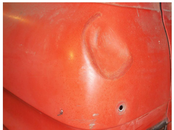
Fig 8. Typical rear corner dent.
