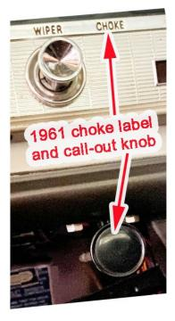
instrument cluster trim plate since the manual coke was replaced with an automatic choke in 1962.
