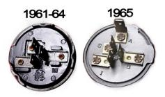
additional contact connected to the circuit that energized the alternator field coils as the engine was cranked.
