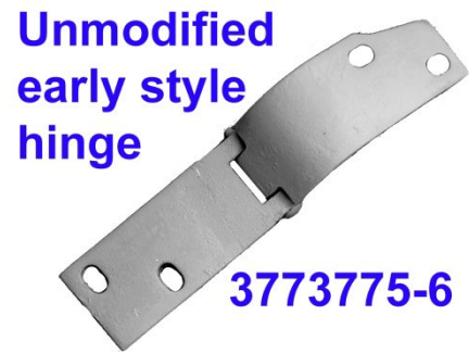
Fig 3. Early style FC rear door hinge
