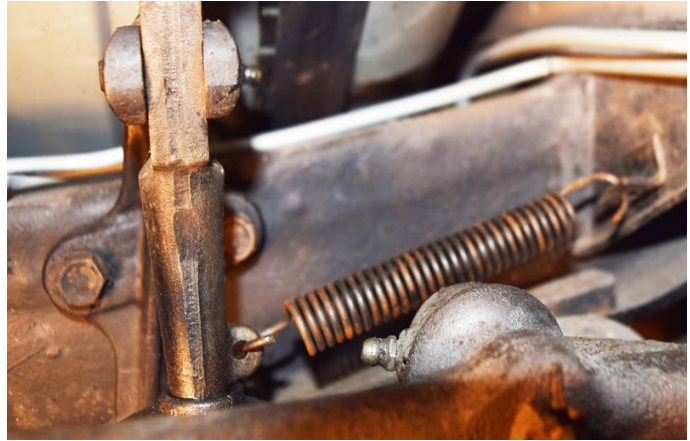
Figure 5. Early design shifter stabilizing spring.
