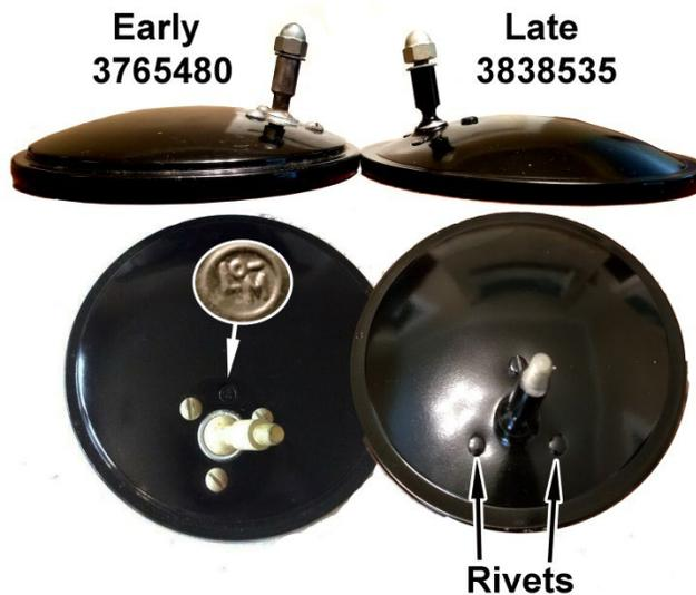
version, and used two rivets and a screw used to secure the mounting bracket. [Thanks to Thomas Pedigo for providing the pictures.]
