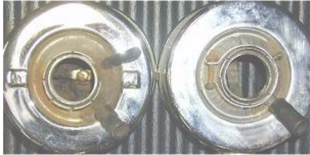
Note slight difference between 1964 on left and 1965-66 Chrome aircleaner on right
