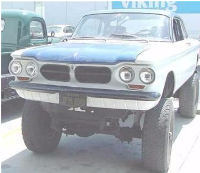
An Early model Corvair converted into a 4X4.
