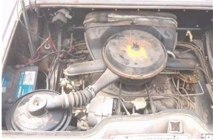
Late model Desert air package. Notice plenum
